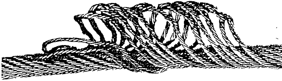
Figure 50. Cable Bird Cage
