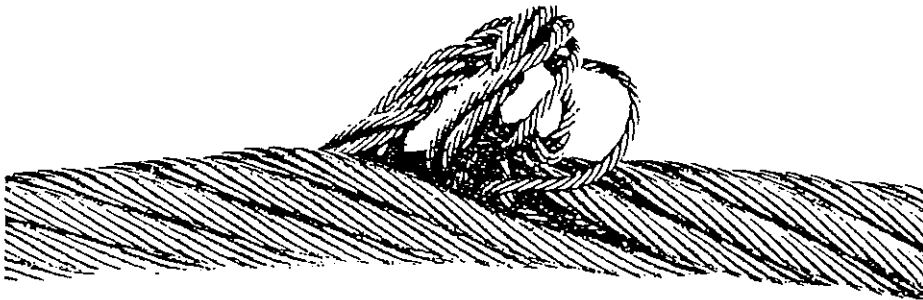
Figure 51. Cable Protruding Core
